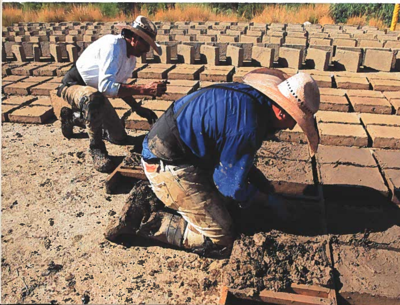
Rafa Esparza and his father, Ramón, making adobe bricks, as part of the performance building: a simulacrum of power , 2014. Courtesy Clockshop, Los Angeles. Photo Jeny Amaya.
